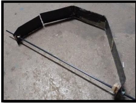
Figure 8.1: Landing Gear Failure after Static Loading Test
